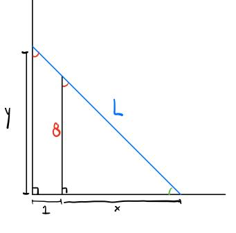
\* Note: INSTEAD OF MINIMIZING THE CENTRY OF THE LADDER L, Let's MINIMIZE L' , THE SQUARE OF THE LENGTH OF THE CADDER CLEARLY, L' 15 MINIMIZED WHEN L IS MINMIZED.
