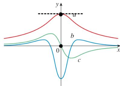
$f''(x) = b$  : GRAPH  $c$  HAS 2 POINTS WHERE TANGENT LINES HAVE SLOPE 0 AND FOR THESE SAME  $x$ -VALUES, GRAPH  $b$  IS 0.
